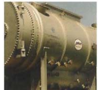
Steam surface condensers
