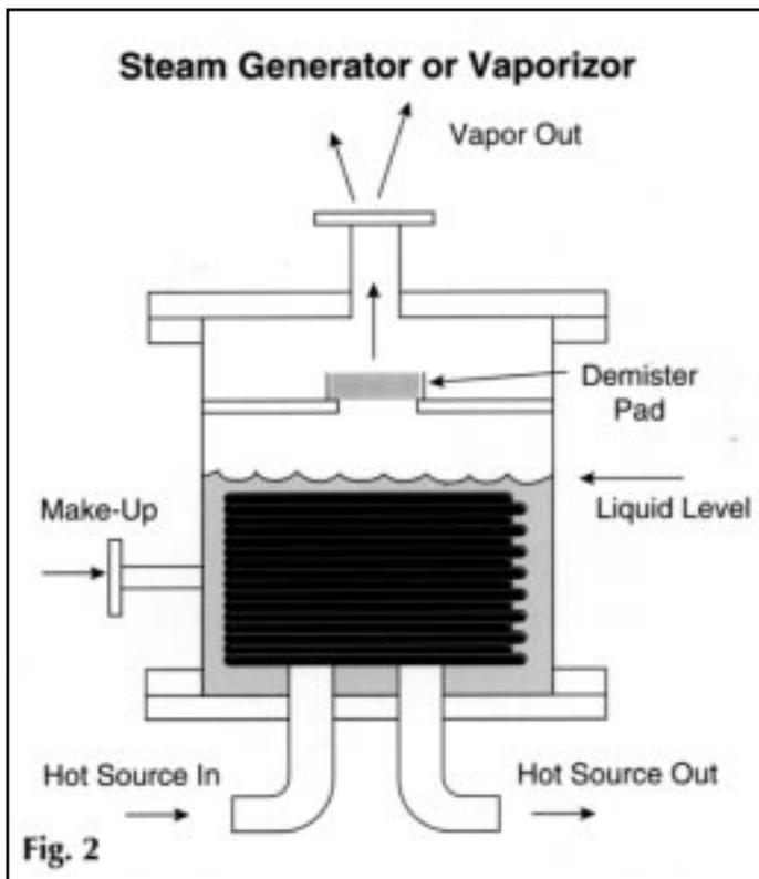
Vaporizer design of a helical heat exchanger for liquid evaporation and droplet disengagement. (Fig. 2)
