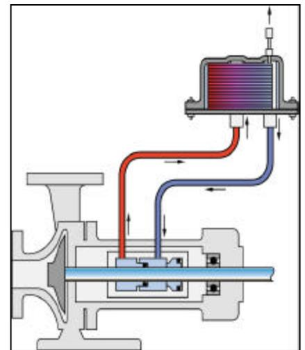
Figure 1. A typical seal cooling arrangement
