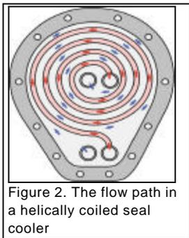
Figure 2. The flow path in a helically coiled seal cooler
