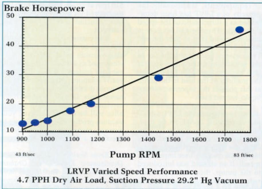
Figure 1. Typical 50 hp LRVP operating at a high vacuum level – note that horsepower requirement drops dramatically as the rpm is reduced while the suction pressure remains constant.
