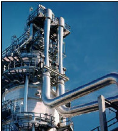
Figure 7. First stage ejectors for CVDU.
