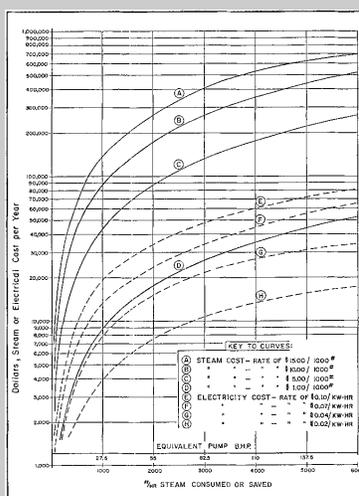
A comparison of approximate costs of steam and electricity. Using these rates, an individual can analyze the cost savings based on the rates that are applicable for his/her locality.
