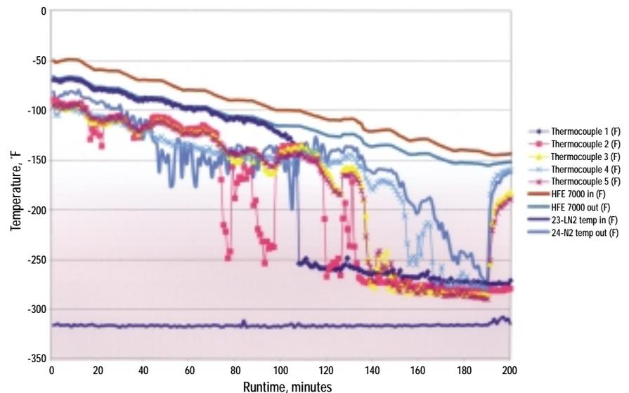
7000 are mixtures. They are composed of a number of different fluids, with each having varied freeze points. Methanol cannot reach the cold temperatures that HFE 7000 can; however, it does perform well at temperatures above  $-130^{\circ}\text{F}$ .
