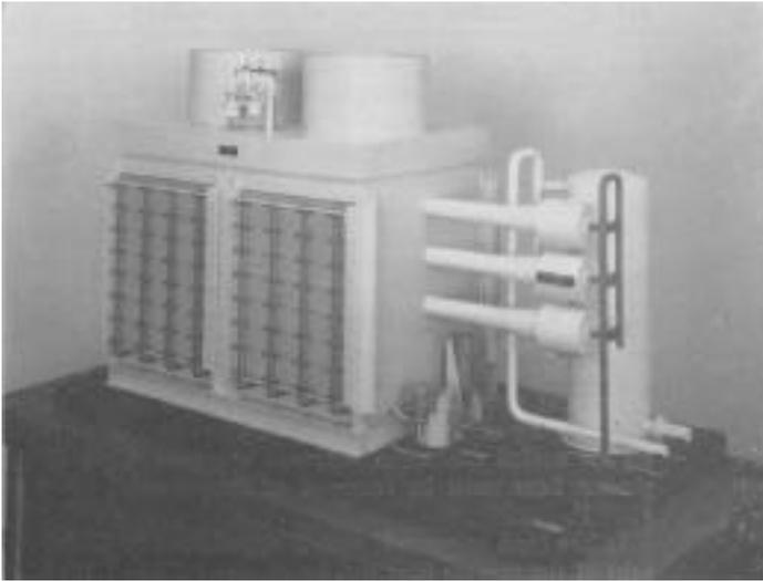
**FIGURE 2-** *This twin cell evaporative cooled steam condenser services a steam vacuum refrigeration system for producing 45°F chilled water. The flash tank and three booster ejectors are shown on the right.*
