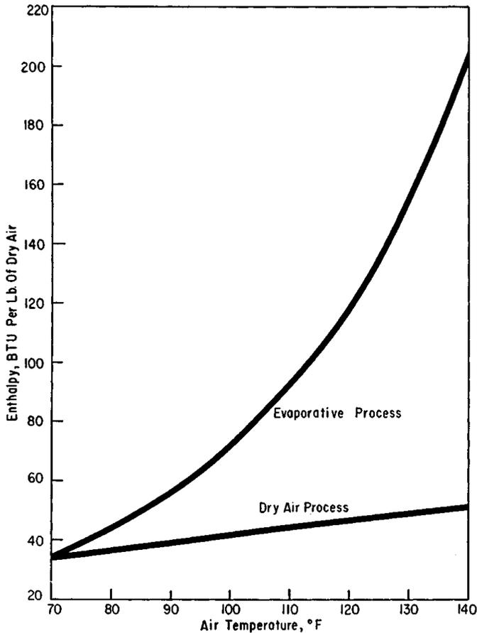
**FIGURE 3-**For an initial wet bulb temperature of 70° F, here is how evaporative cooling compares with dry air cooling.
