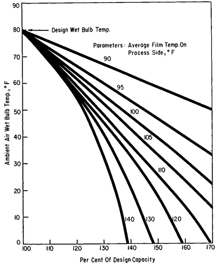
**FIGURE 4-**Typical performance for an evaporatively cooled heat exchanger with constant-speed fixed-pitch induced flow fan.
