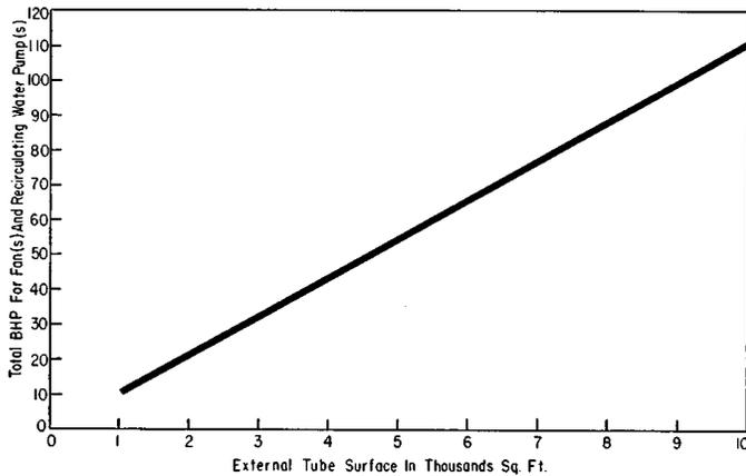
**FIGURE 6-** Typical maximum horsepower requirements for evaporatively cooled exchangers. By increasing the cooling surface in a particular application the fan power requirements can be reduced to some suitable level.
