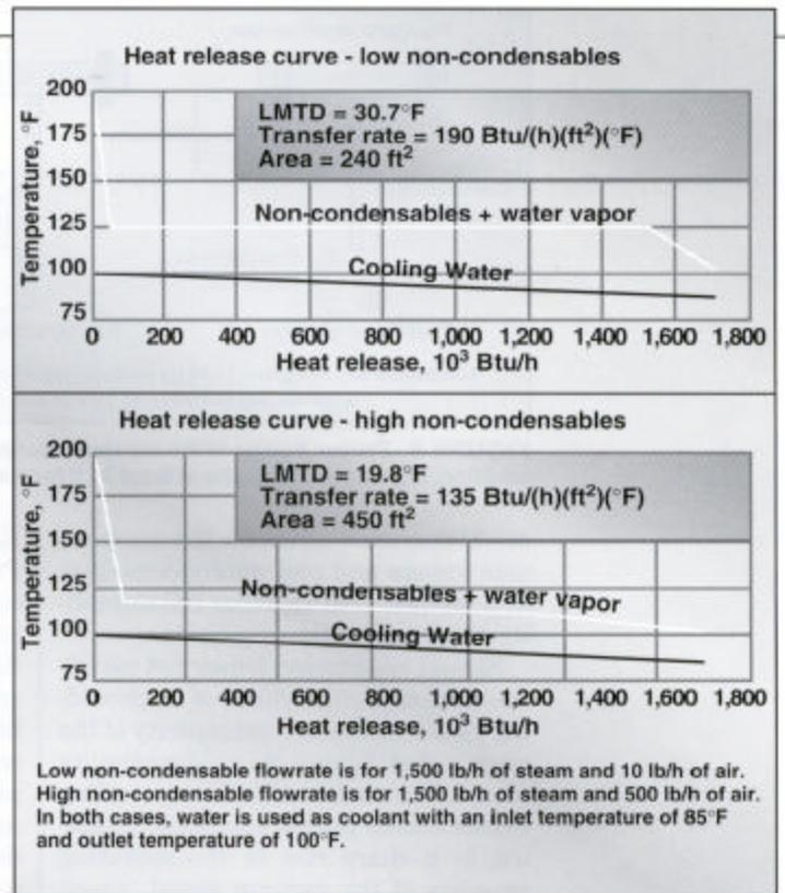
**FIGURE 4.** High non-condensable loadings can cause poor LMTD, reduce heat transfer rates and require greater surface areas
