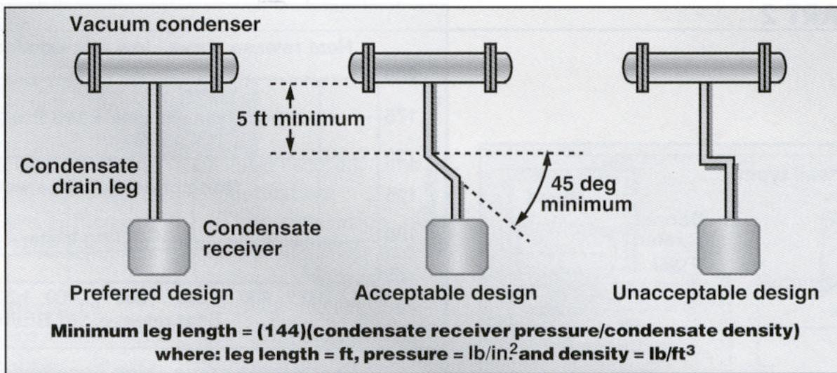
**FIGURE 5.** Proper design of the condensate drain leg must consider these factors. In addition, leg length should be at least 34 ft for water and 45 ft for hydrocarbons
