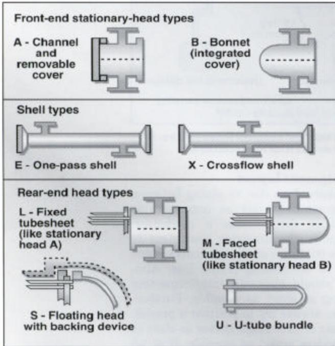
**FIGURE 3.** Condenser design allows for a "mix-and-match" of geometries that follows standard TEMA designations
