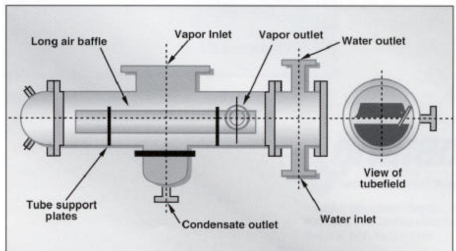
**FIGURE 2.** The elements of a typical vacuum condenser are shown for a crossflow shell unit that makes use of a long baffle
