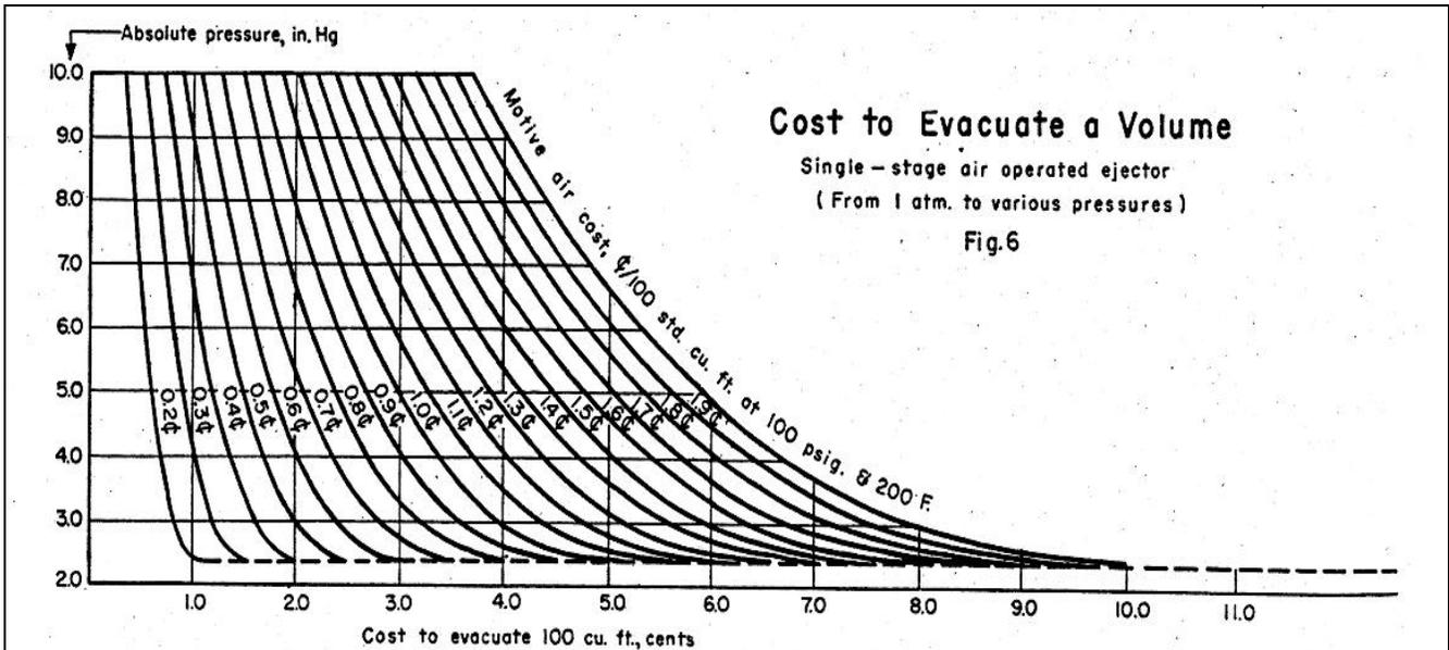
stage 100 psig. air compressor with a capacity of slightly more than 37.5 scfm. is found to be approximately 22 bhp./100 scfm. delivered. With this value and the fuel costs listed above we can enter the other tables of the "Compressed Air Data" book and find the power costs for running the compressor on the various fuels:
