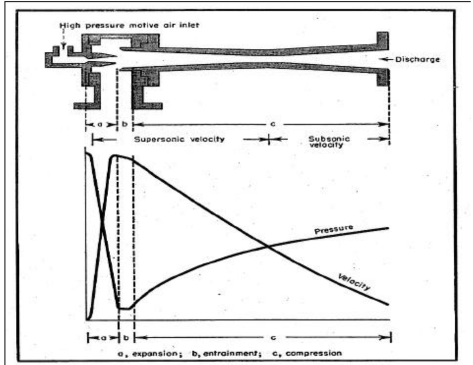
Fig. 1 - Ejector nozzle converts air pressure into velocity and the diffuser converts velocity back into pressure.
