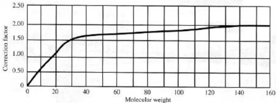
Figure 5. Molecular weight correction factor to convert different vapors to water vapor equivalent.
