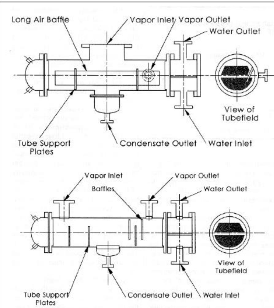
Figure 7. Vacuum condensers typically used as condensers or precondensers: Tema "X" and "E" shells
