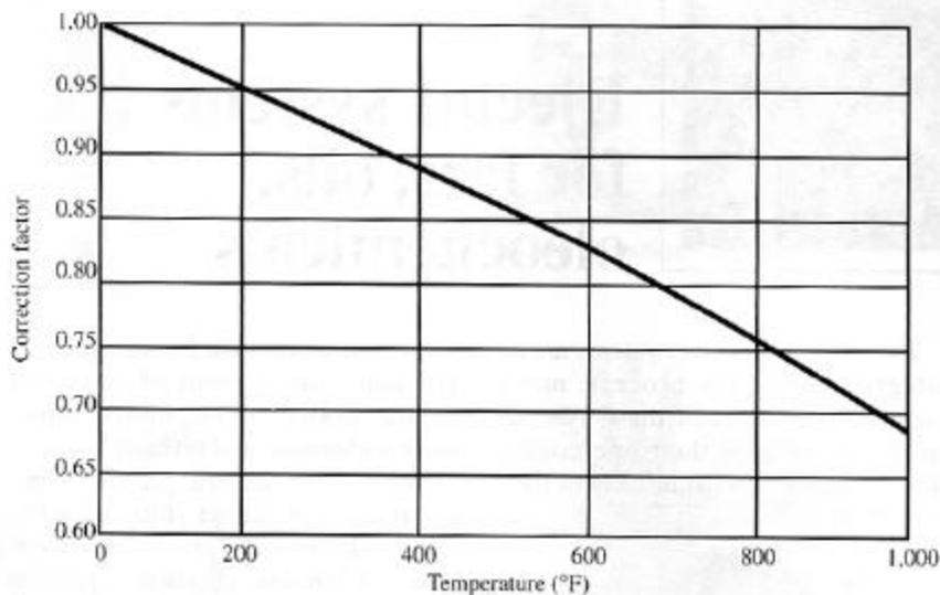
Figure 4. Temperature-correction factor curve for converting different temperatures to 70°F equivalent load.
