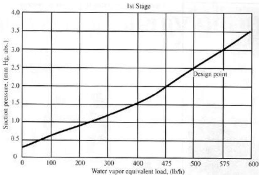
Figure 3. Ejector performance curve for first stage of deodorizer ejector system. (Water vapor equivalent load is on the abscissa and suction pressure maintained by the ejector is shown on the ordinal. Minimum motive steam pressure, 140 psig at 450°F; maximum pressure discharge, 13 mm Hg absolute).
