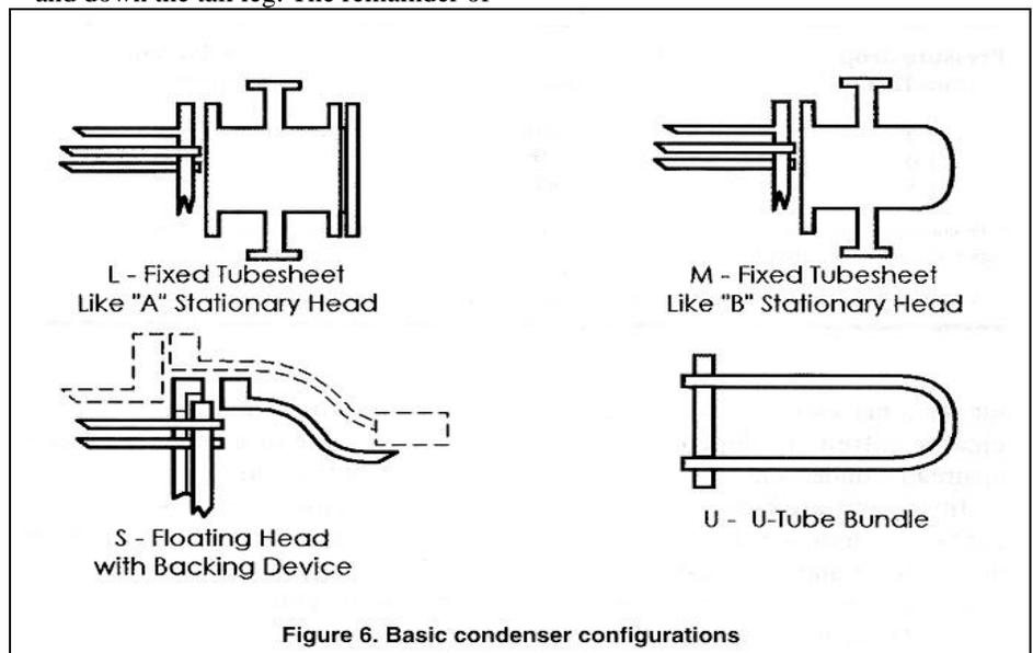
**Figure 6. Basic condenser configurations**
