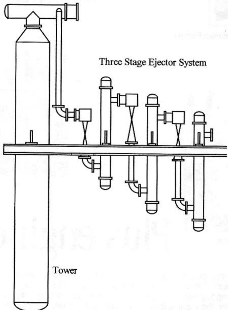
Figure 11. Precondenser mounted atop vacuum column
