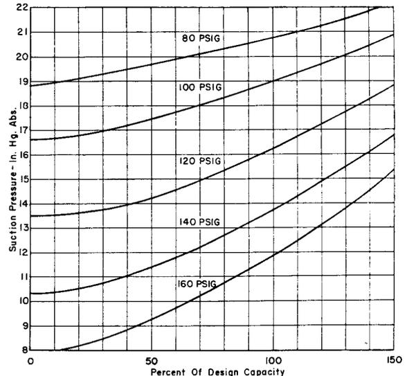
FIGURE 2—The capacity of a throttling ejector is a function of both the suction pressure and the motive steam pressure. Basic design here is 100 psig.
