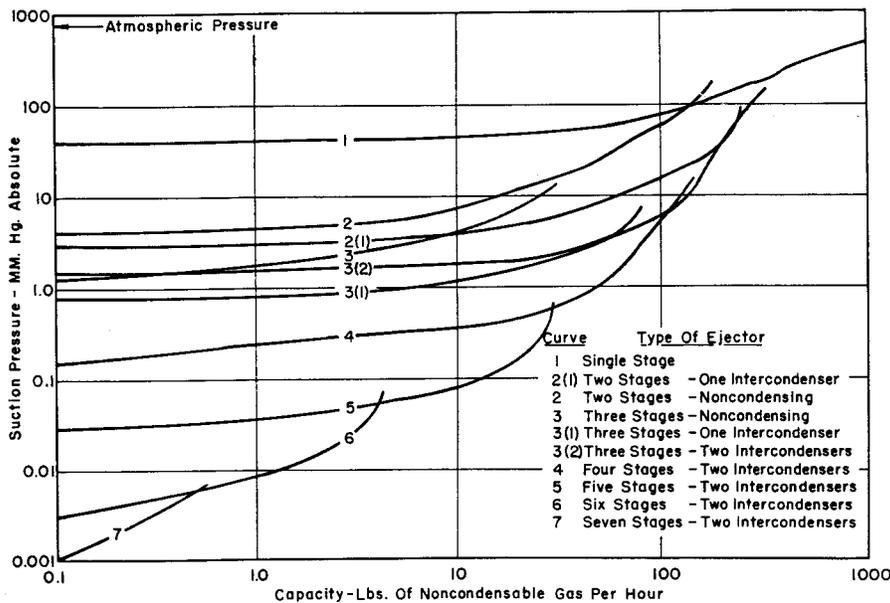
FIGURE 3—A wide range of pressures can be achieved by using various combinations of ejectors and condensers. The same steam consumption is used for each design here.
