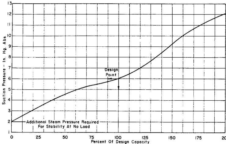
FIGURE 1—For a fixed-capacity ejector, increasing the steam pressure will not increase the capacity.
