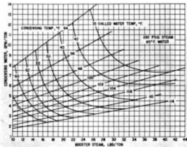
Fig 4: Utility requirements for steam vacuum refrigeration systems.
