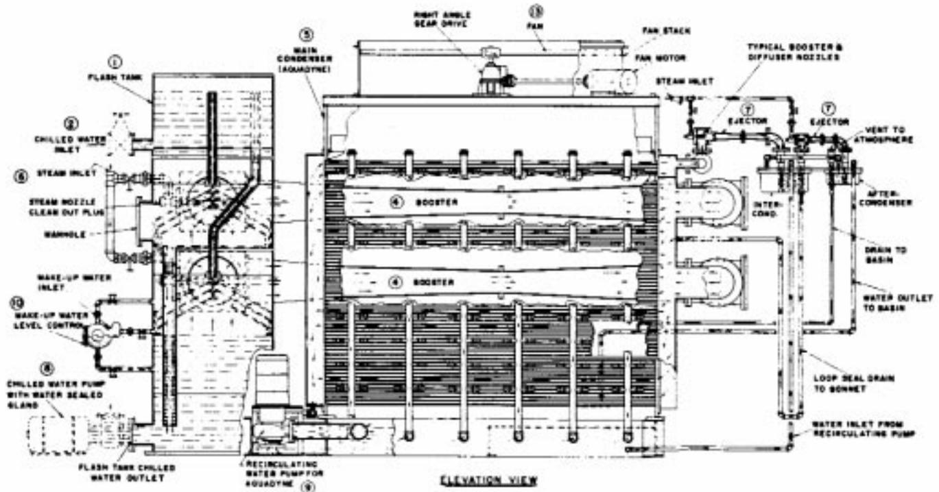
Fig 3: Steam vacuum refrigeration system with evaporative type condenser.
