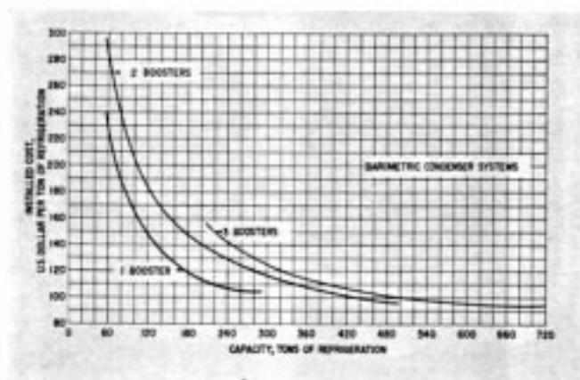
Fig 5: Installed cost per ton, barometric systems using one, two or three boosters.
