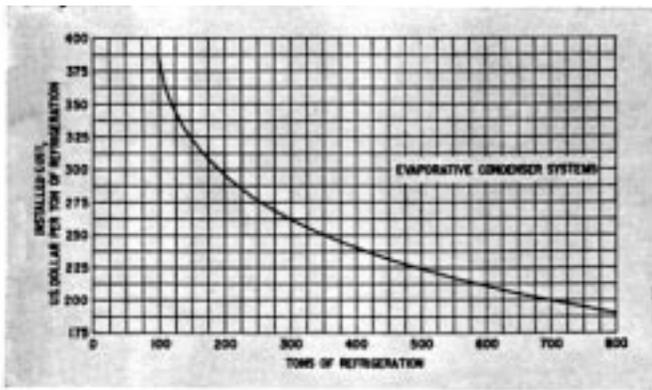
**Fig. 7:** Installed cost per ton for systems with evaporative condensers.
