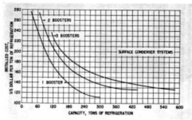
Fig 6: Installed cost per ton, surface condenser systems, using one, two or three boosters.
