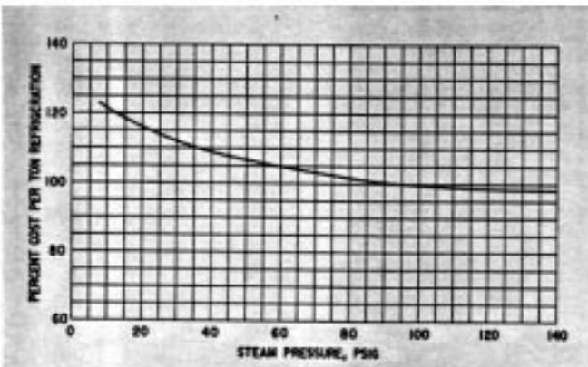
**Fig. 9:** Cost correction factors for various steam pressures.
