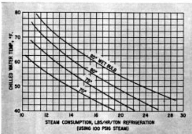
**Fig. 8:** Steam Consumption in pounds per hour per ton of refrigeration.
