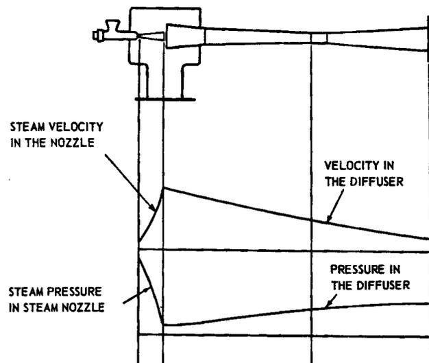
*Figure 1. Conversion of steam pressure into velocity in the steam nozzle and conversion of velocity into pressure in the diffuser.*
