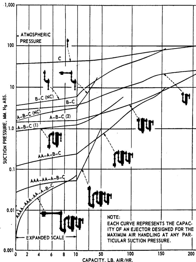
Figure 3. Plot of production plant ejectors.
