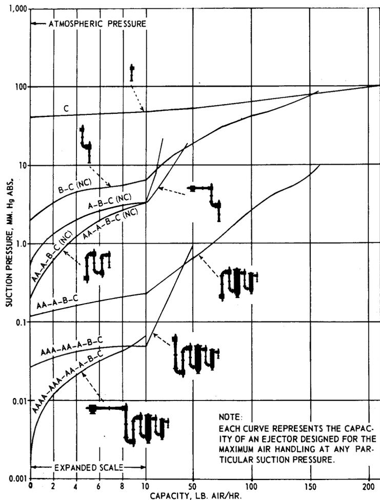
Figure 4. Plot of pilot plant ejectors.
