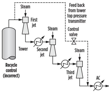
**FIG. 6.** The vacuum system’s recycle pressure control caused the tower pressure to fluctuate when it was put into service, but a P&ID review determined that the recycle line was installed correctly.
