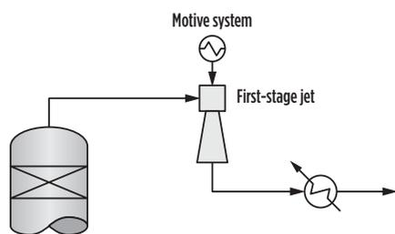
FIG. 3. Extra steam to the vacuum heater overloads the first-stage jet.
