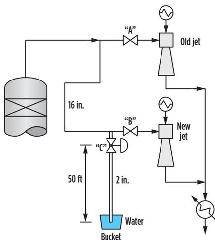
FIG. 4. Commissioning the spare first-stage ejector.
