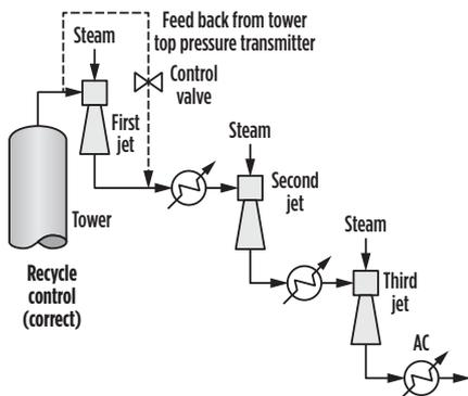
**FIG. 7.** A larger pressure differential allows the sizing of a smaller line and control valve.
