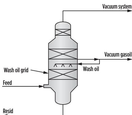
FIG. 2. Wash oil protects the grid from coking.
