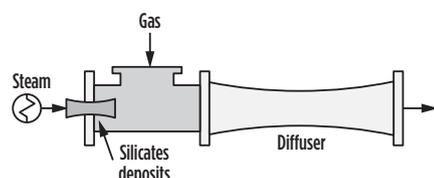
FIG. 5. Silicate fouling is a possible cause of poor ejector performance in refineries.
