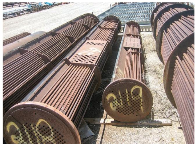
FIG. 6. A maintenance yard filled with failed bundles.
