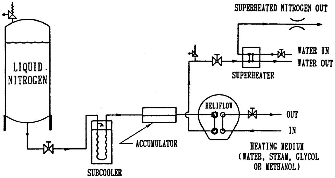
Fig. 2 Flow schematic of LN<sub>2</sub> vaporization test apparatus
