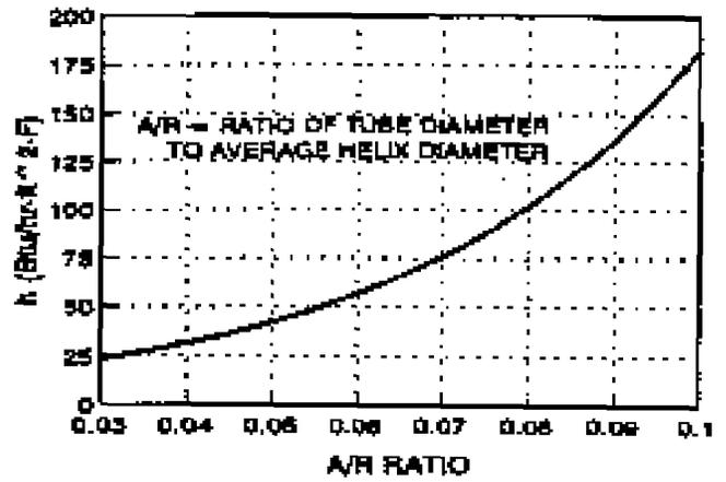
Fig. 6 Effect of coiled-tube geometry on the boiling coefficient
