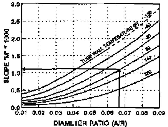
Fig. 7 Determination of Reynolds coefficient "M"
