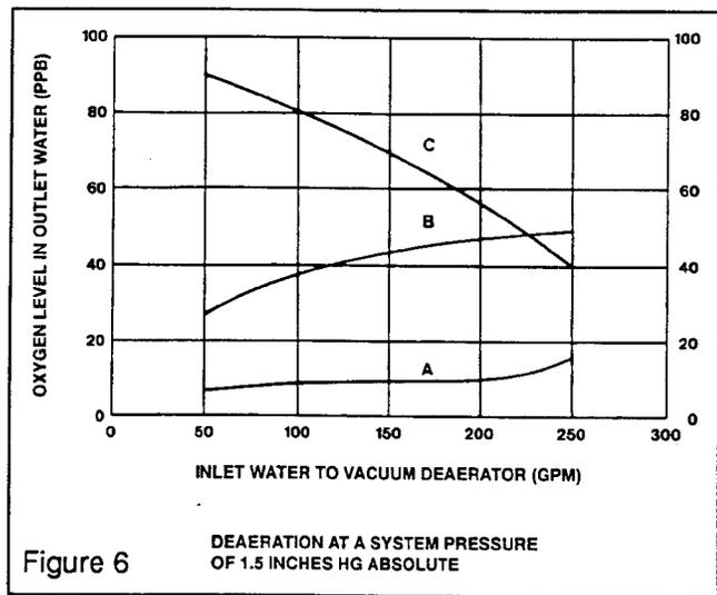
internal pressure of 1.5 inches Hg absolute the steam flow can be insufficient to provide adequate deaeration unless the engineering design parameters are adjusted. In the case shown in Figure 6, packing "B" is obviously unacceptable, while packing "A" gives results in the 8 - 10 ppb range.
